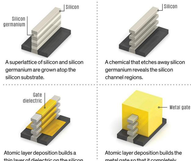
thin layer of dielectric on the silicon channels, including on the underside. metal gate so that it completely surrounds the channel regions.
