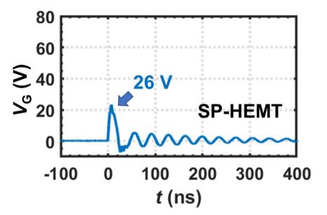
Dynamic gate voltage ICeGaN offers "extreme robustness" against dynamic voltage overshoots on the gate terminal <sup>[1].</sup>
