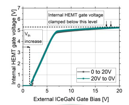
The internal gate of the transistor is clamped to 6 V even when the external gate voltage is increased to 20 V.
