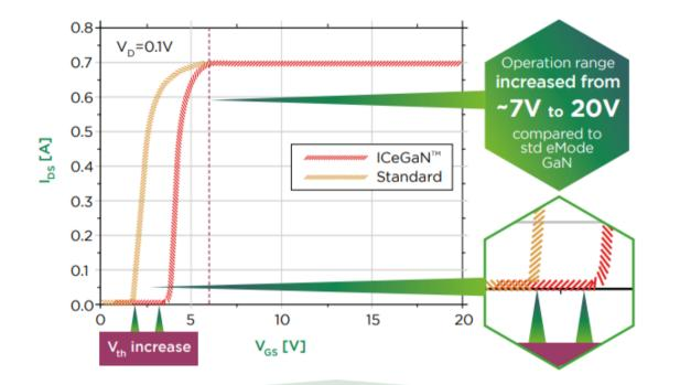
The threshold voltage,  $V_{th}$ , of an ICeGaN<sup>TM</sup> device is around 2.8 V compared to 1.6 V for the conventional counterpart.
