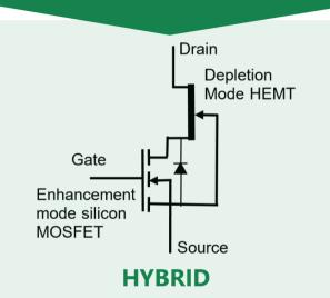
Schottky gate depletion mode HEMT in a hybrid integration with a silicon low-voltage MOSFET
